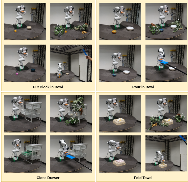
Fig. 9: Tasks considered for the real robot experiments. In clockwise direction: original task, with distractors, with camera occlusions, and with color changes.
