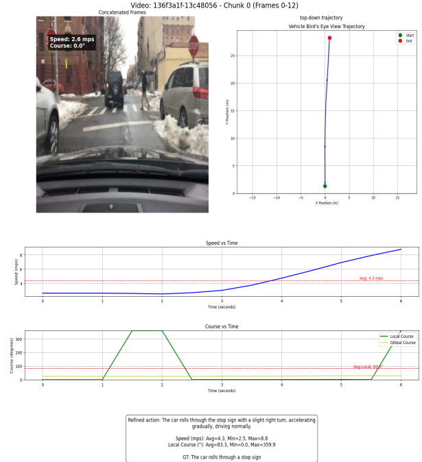
(a) Starting with the label “The car accelerates slowly”, we can augment with additional information from the vehicle’s states to get the label “The car rolls through the stop sign with a slight right turn, accelerating gradually, driving normally.”
