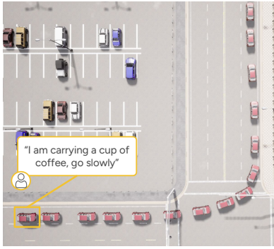
(a) When prompted with “I am carrying a cup of coffee, go slowly”, SteerVLA predicts cautious meta actions and executes the turn at a reduced speed.
