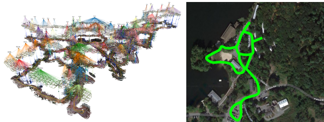
Fig. 1. Left : A kilometer-scale 3D scene graph with 314 objects, 15944 places, and 124 regions. Right : Scene graph extent on overhead image.
