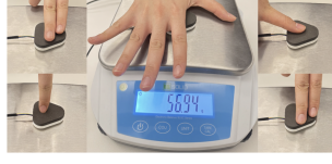
(b) Different modes of contact for data collection; Two fingers laid flat (top left), index fingertip (bottom left), palm (middle), one finger laid flat (top right) and two fingers pressing at an angle to emulate a combination of both normal and shear forces
